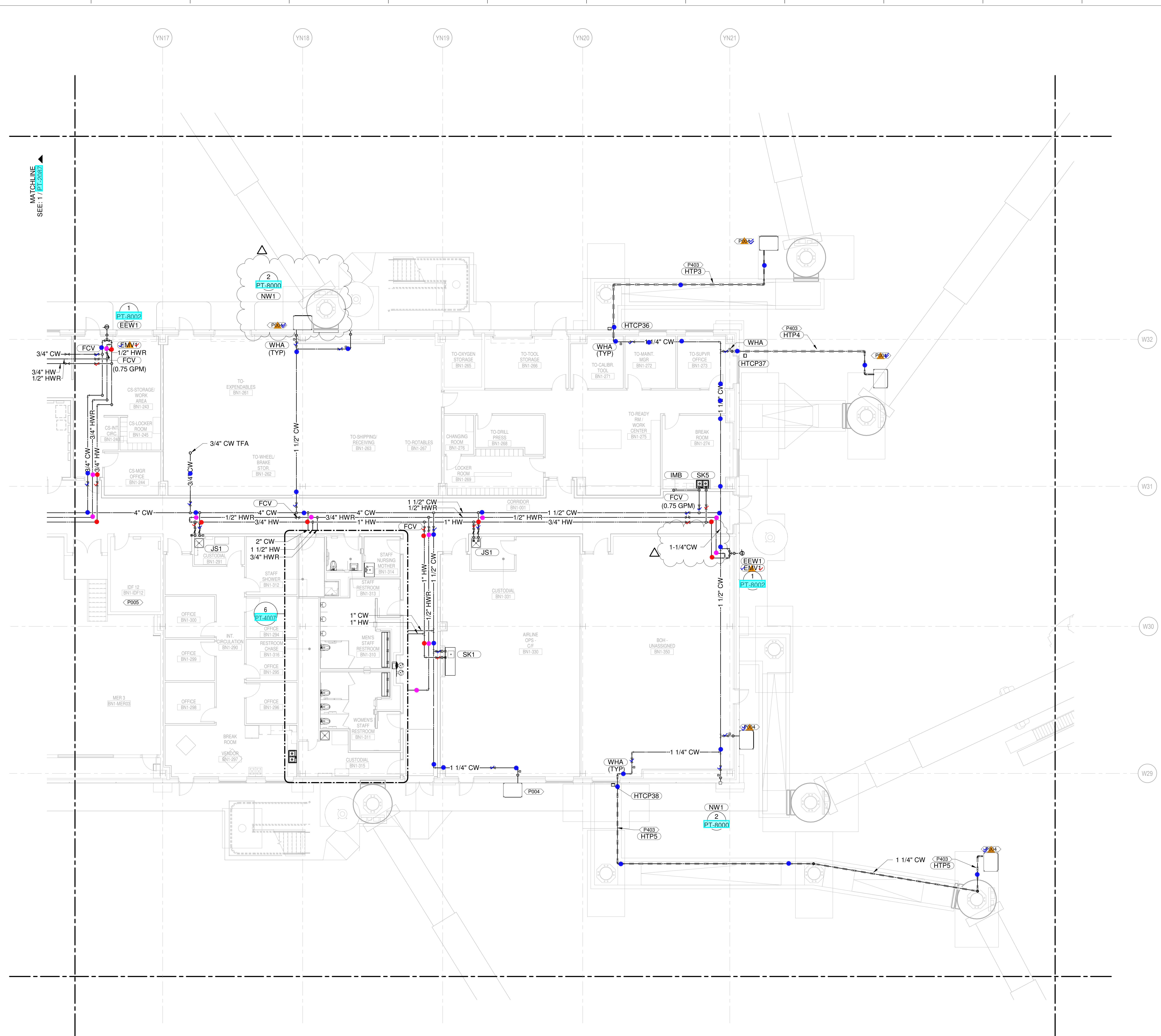
1 LEVEL 1 - ARRIVALS WATER & GAS PART PLAN T88 SCALE: 1/8" = 1'-0"
