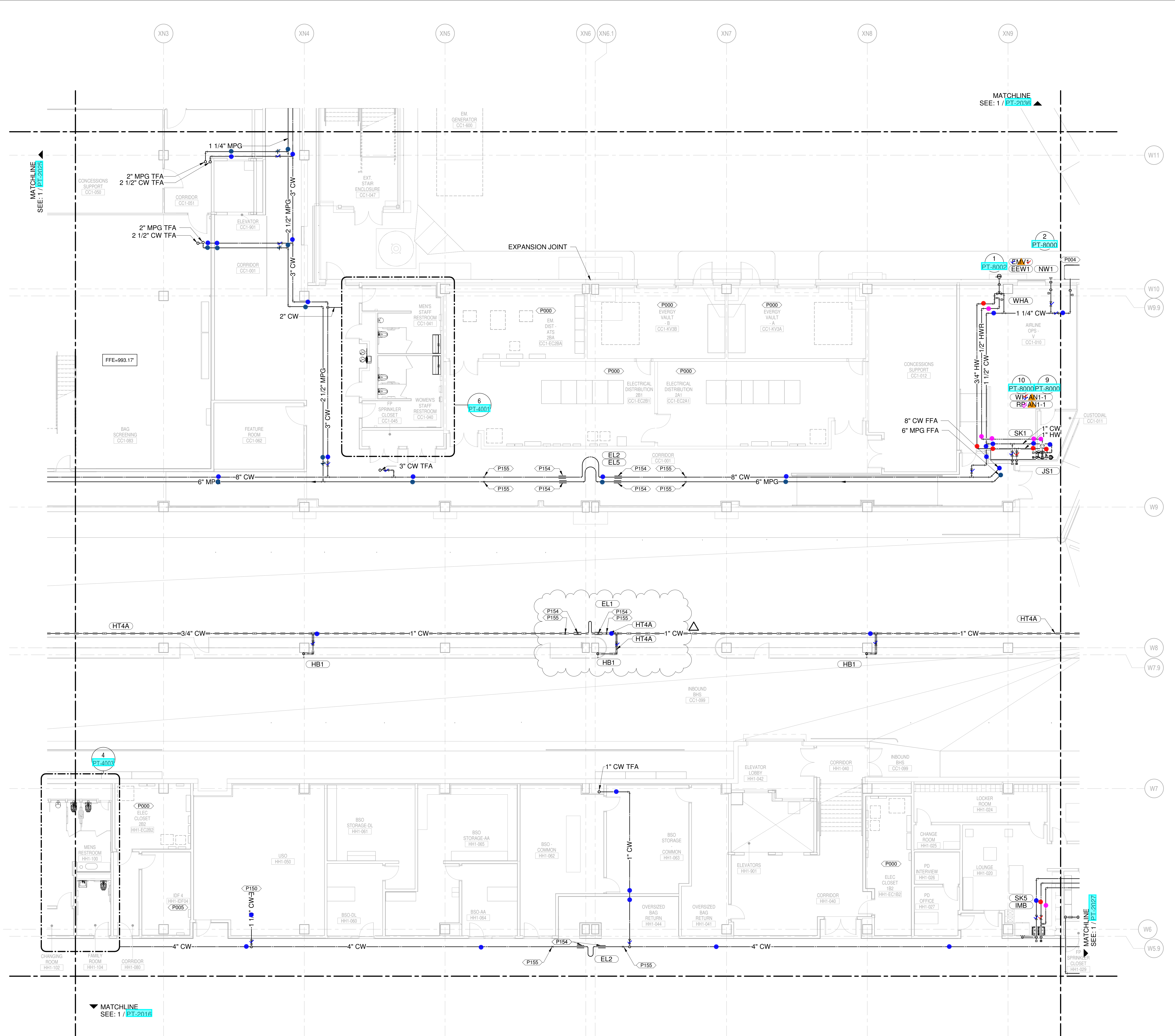
1 LEVEL 1 - ARRIVALS WATER & GAS PART PLAN T26 SCALE: 1/8" = 1'-0"
