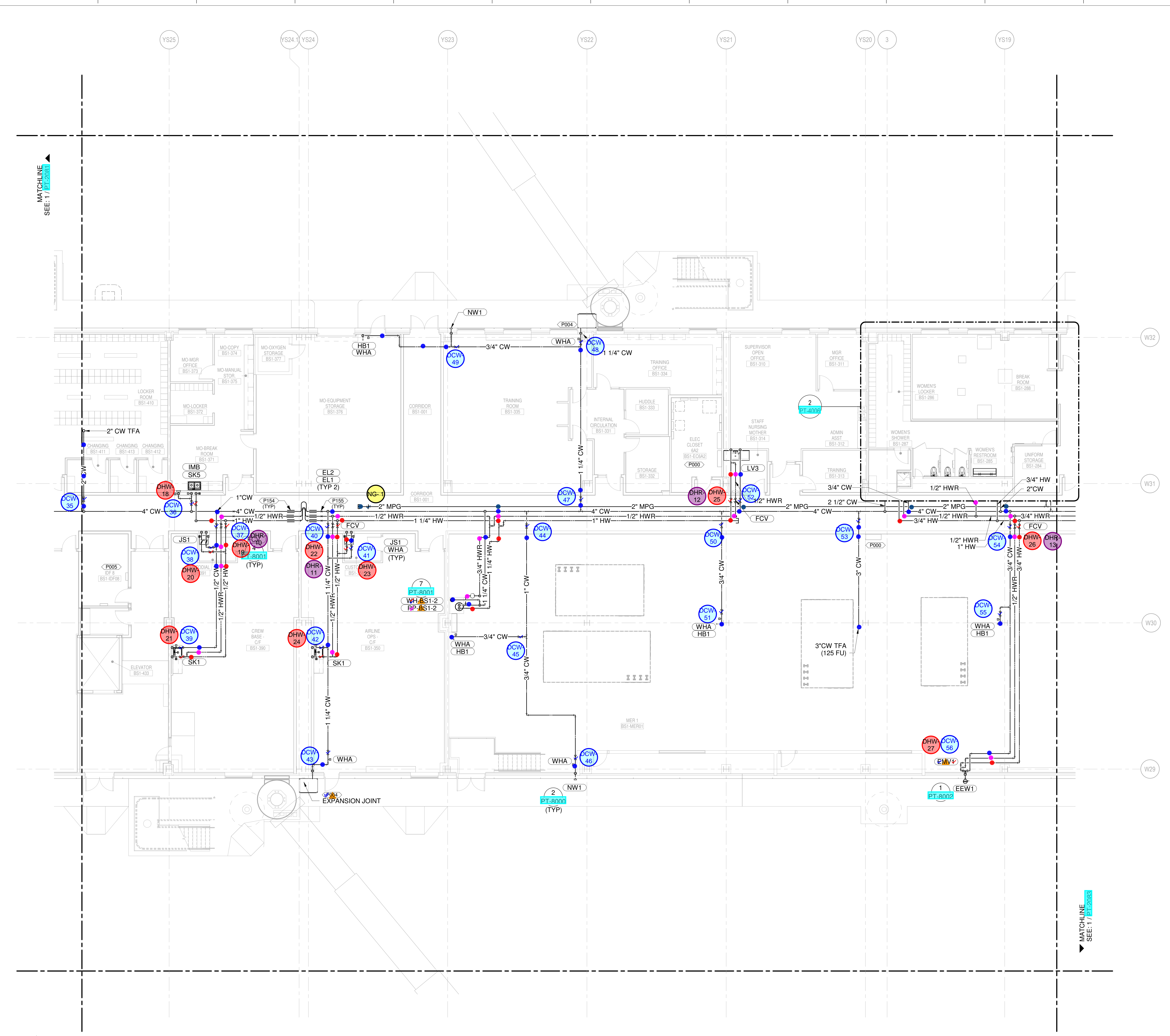
1 LEVEL 1 - ARRIVALS WATER & GAS PART PLAN T82 SCALE: 1/8" = 1'-0"
