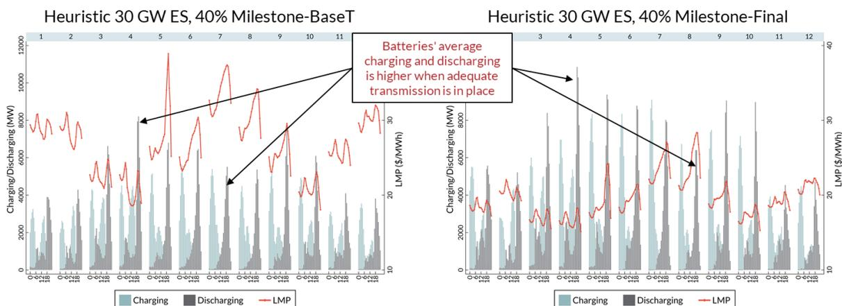
**Figure EA-65: Monthly diurnal average of battery charging and discharging in the heuristic scenario of the energy storage sensitivity, with base transmission (BaseT, left) and RIIA transmission solutions (Final, right)**
