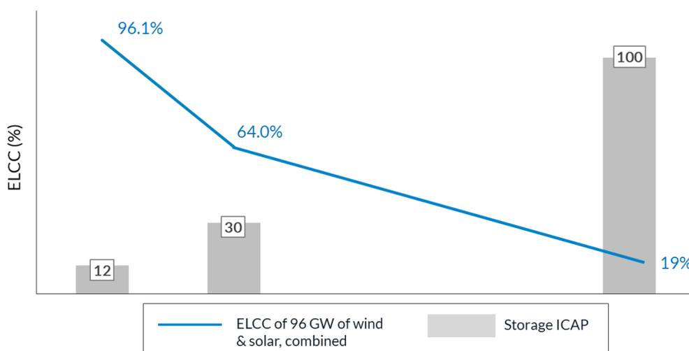
**Figure RA-32: ELCC of storage as the penetration of storage increases**
