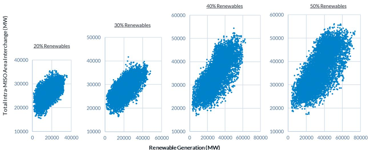
**Figure EA-21: Intra-MISO interchange from RIIA 20% to 50% milestones. The increasing upper limit of the cloud of points indicates increased interchanges, while the increasing height of the cloud indicates increased variability**
