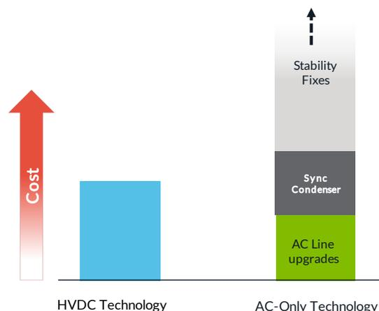
To port power from wind-rich zones located in weak-area, building a VSC- HVDC line into those weak-areas may be more economical than incrementally installing a combination of AC transmission lines with many synchronous condensers and mitigating the small signal stability issues created by installing the rotating masses of those synchronous condensers
