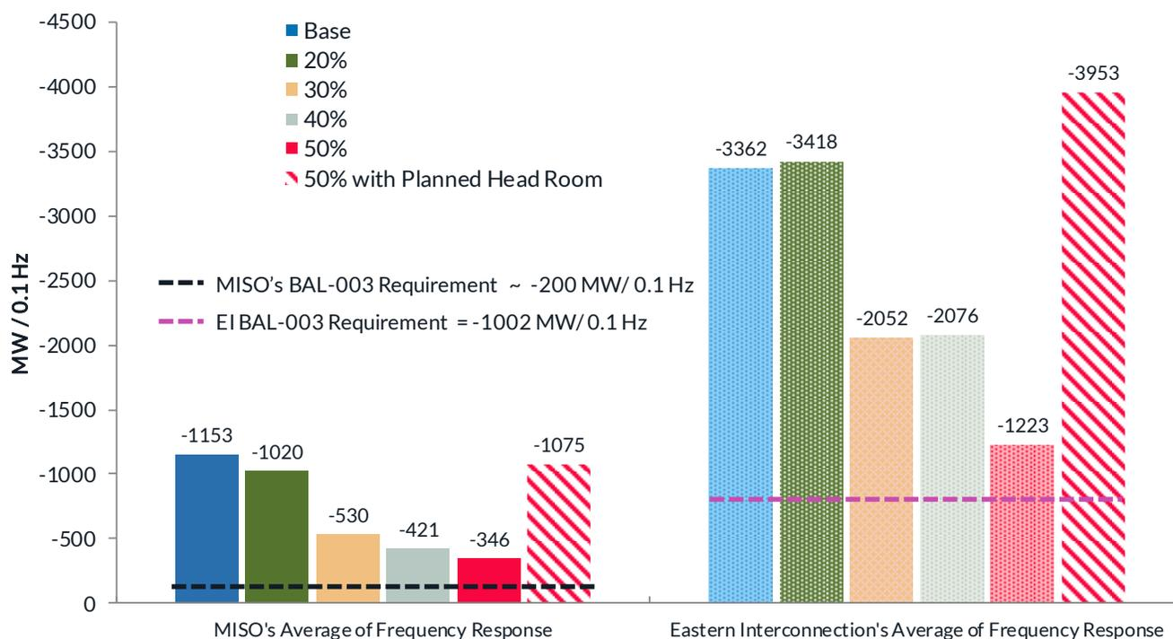
Negative sign in Primary Frequency Response value indicates under-frequency event. Average performance in absence of planned headroom remains high largely due to good performance in Peak Snapshot and smaller generator (MW) trip events.
