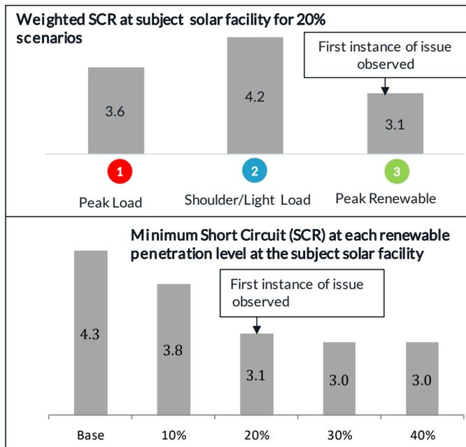
Undamped voltage oscillations in low SCR area fixed by tuning the gains of solar plant A
