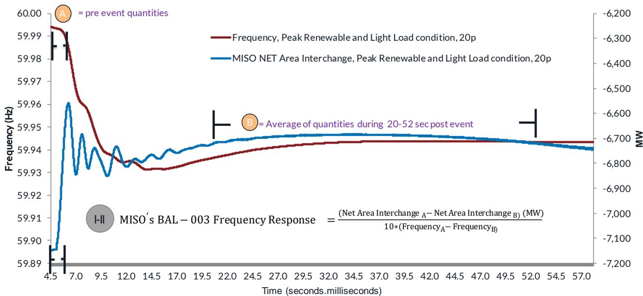
Figure TA-28: MISO's BAL-003-1 obligations are calculated based on Net Area Interchange and Frequency profile
