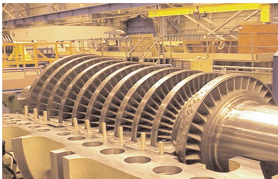
Figure 9. Dense Pack redesign of a single-flow high-pressure rotor
