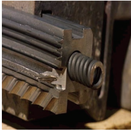
8. Sealed up tight. Installing a new brush seal (left) and brush-tip seal (right) significantly reduced steam seal leakage within the turbine of Northport Unit 3. Courtesy: TurboCare Inc.
