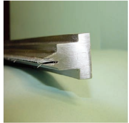
8. Sealed up tight. Installing a new brush seal (left) and brush-tip seal (right) significantly reduced steam seal leakage within the turbine of Northport Unit 3. Courtesy: TurboCare Inc.
