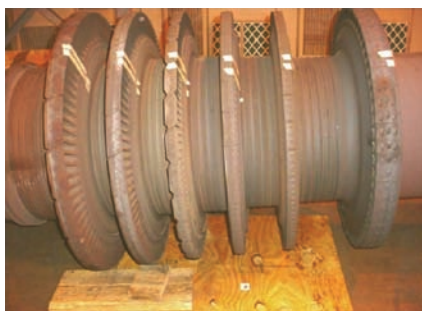
5. You make the call. Compare Labadie Unit 3 and 4's new and old high-pressure (HP) turbines. The old HP section (left) has two fewer rows than the new one (right). Testing found the new design to be 7% more efficient. Courtesy: AmerenUE
