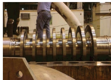
5. You make the call. Compare Labadie Unit 3 and 4's new and old high-pressure (HP) turbines. The old HP section (left) has two fewer rows than the new one (right). Testing found the new design to be 7% more efficient. Courtesy: AmerenUE
