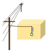
Example C: The drawing below represents a 69kV primary overhead line, a small substation, a 34kV overhead cable providing service to a customer, and a meter installation including a potential transformer, all associated with a Large Primary Service customer.
