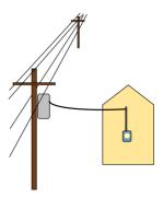
Example B: The drawing below represents a 12.47kV primary overhead line, a 12.47kV overhead cable providing service to a customer, and a meter installation including a potential transformer, all associated with a Small Primary Service customer.
