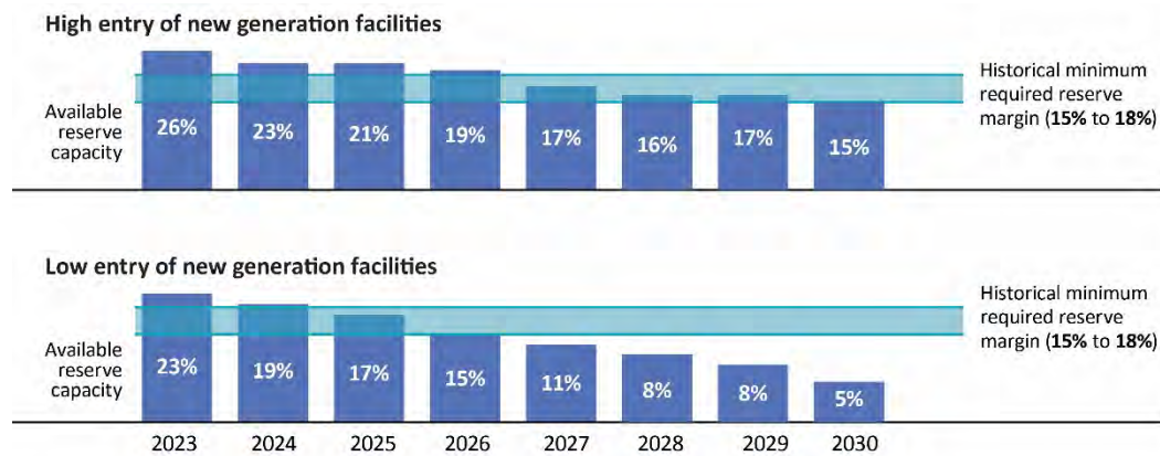
FIGURE 3-5 PJM projects available generating capacity could decline below reserve levels within a few years
