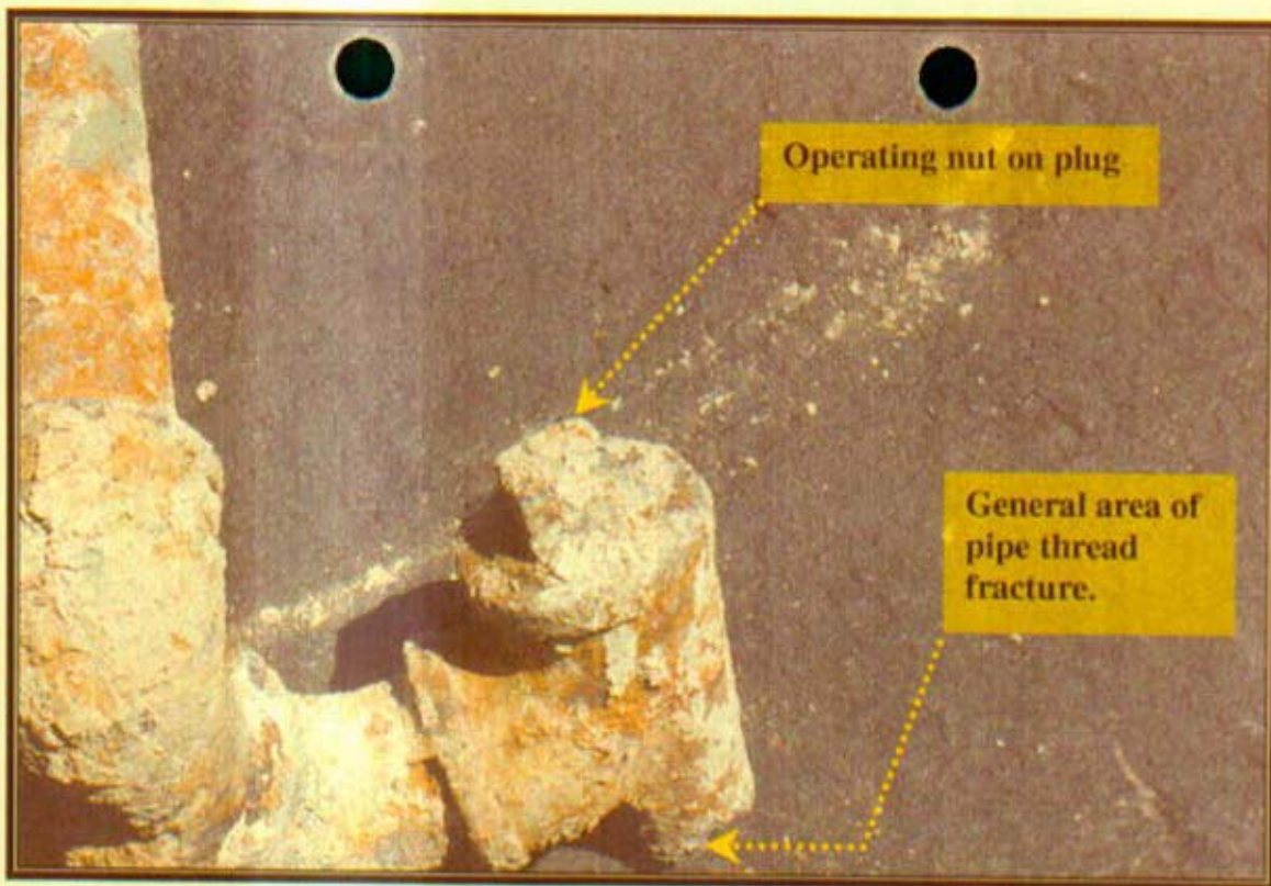
Photograph 1 View of the top side of the tapping tee and attached piping.
