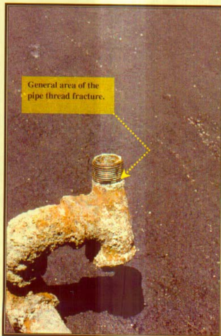
Photograph 4 View of the tapping tee with the section of fractured pipe threads placed on top of the tapping tee. NOTE: The tapping tee and attached pipe components were actually oriented 180° from the position shown.
