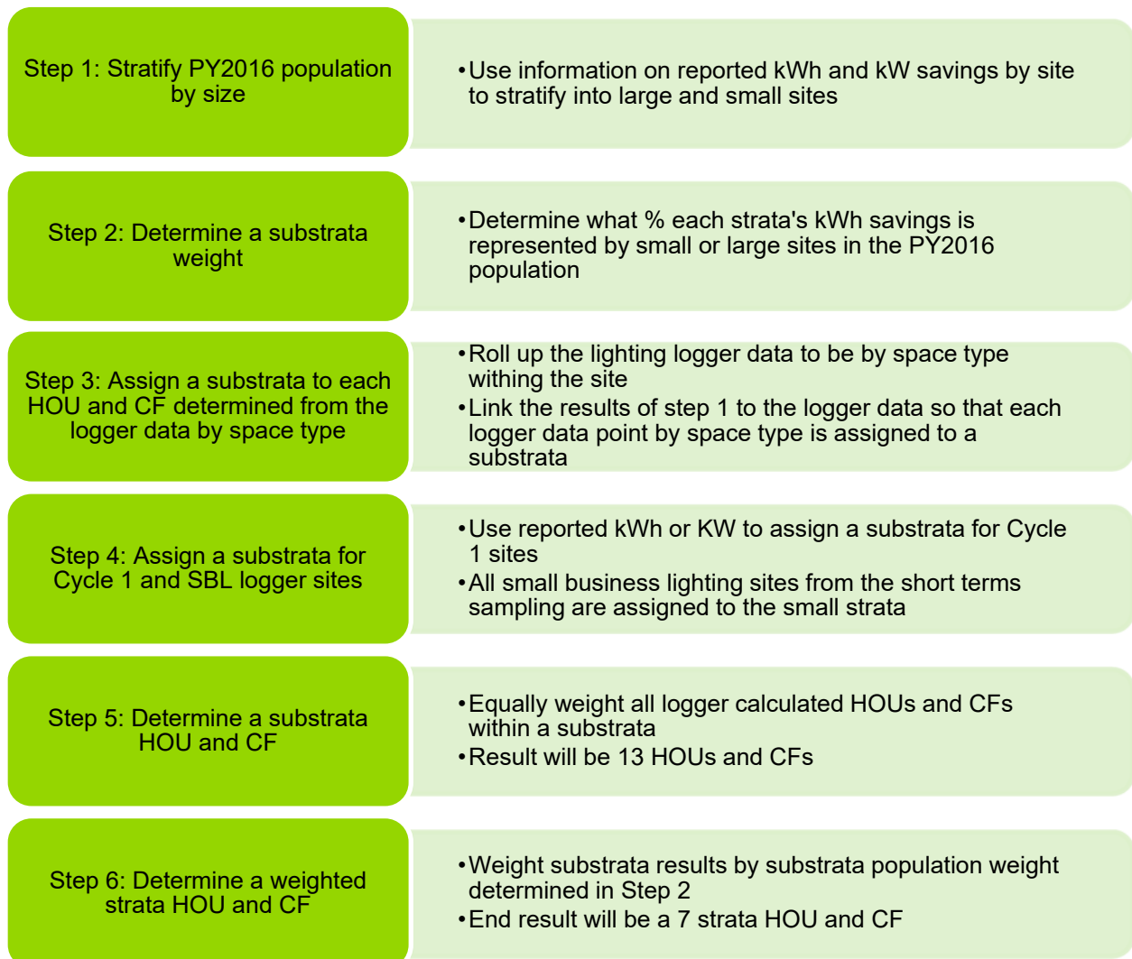
Figure D-1. Methodology for Determining HOU and CF from Logger Data
