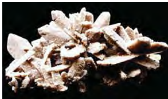
Figure 2-6 – Mixture of \text{CaSO}_3 and \text{CaSO}_4 Crystals (under magnification)
