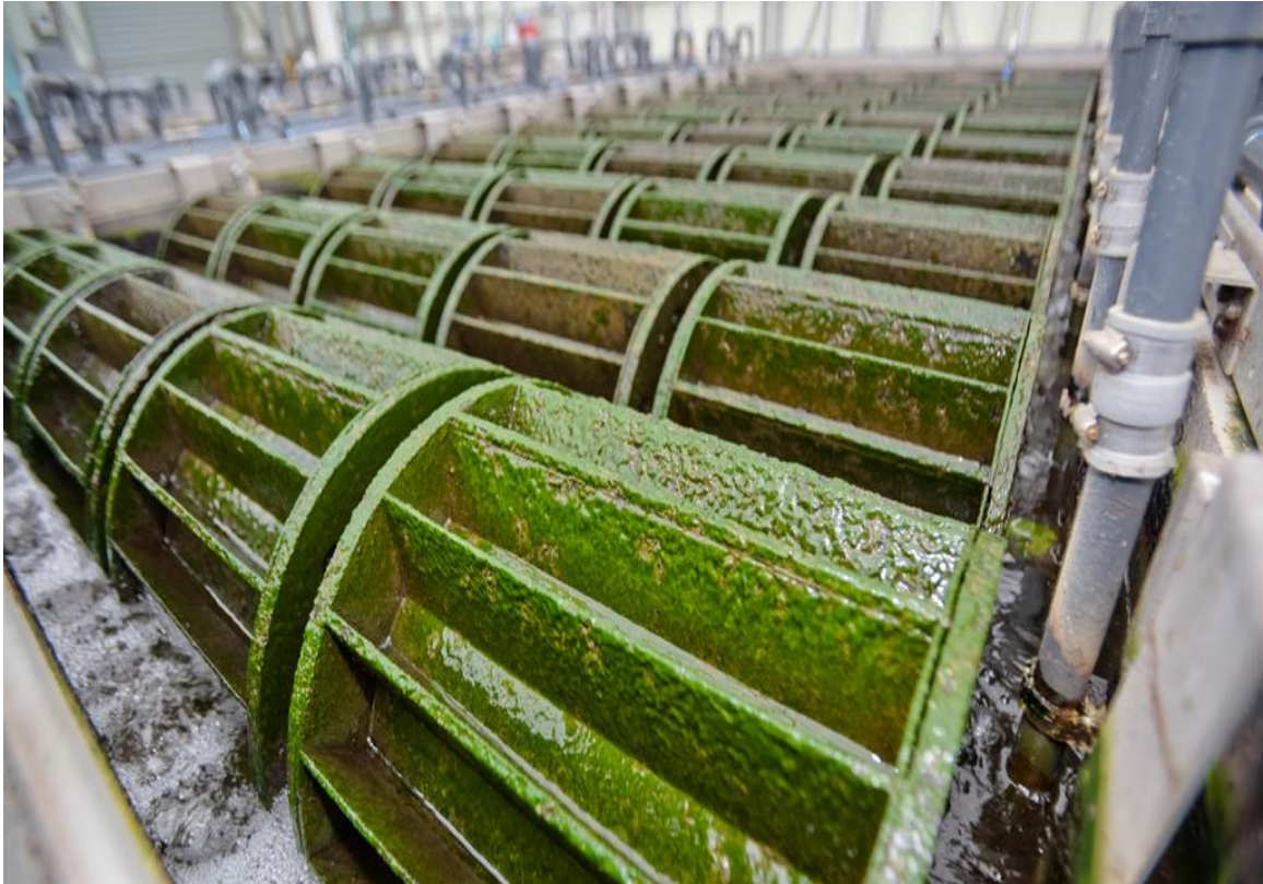
1 2 Multiple Algae Wheels ® running in parallel, algae growth on fins and aeration piping 3
